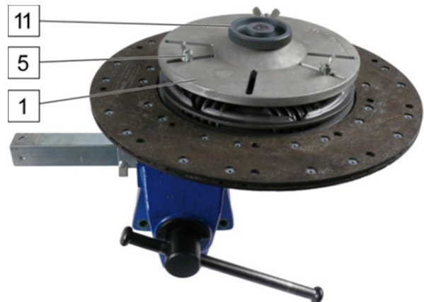
Fig. 5: Installing the fixing plate
